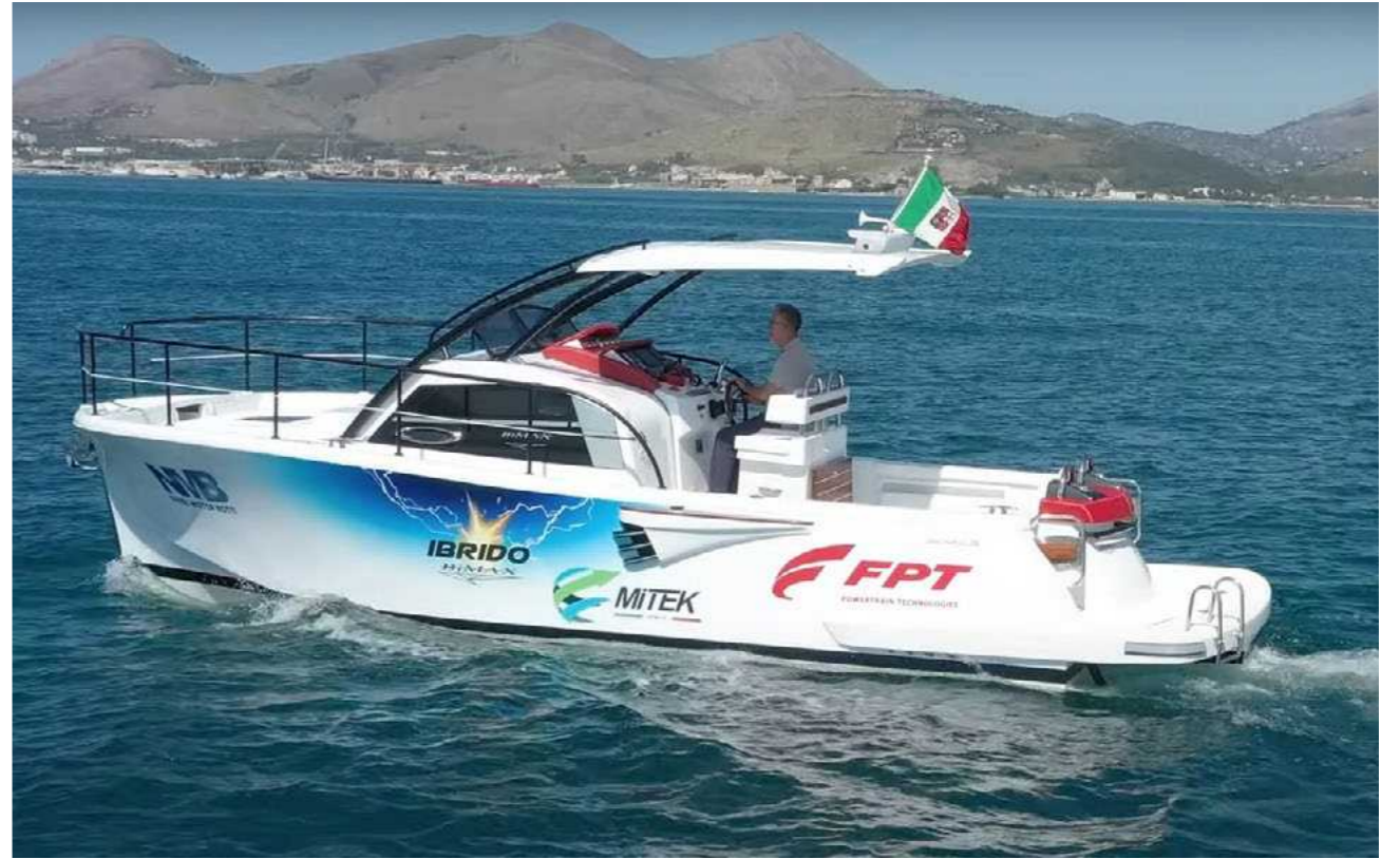
PARALLEL HYBRID WITH INTEGRATED ELECTROMAGNETIC CLUTCH: FPT motor + Mitek inboard motor 7 kWh
