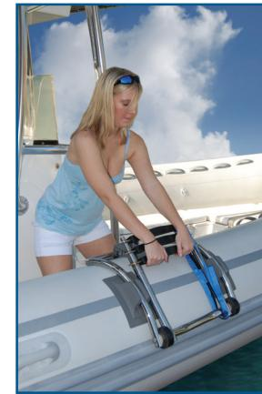
4. Using the step portion of the ladder, pull the hoop out of the snaps.
