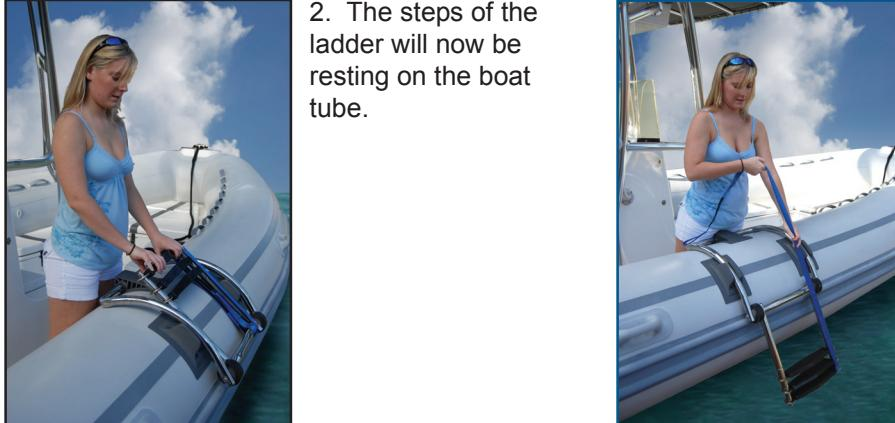
2. Lower the steps into the water, using the strap.
