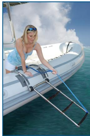
1. Pull the steps out of the water, using the strap.
